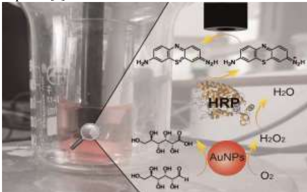
Fig. 8. Schematic illustration of the colloidal AuNPs-based electrochemical detection system [8].
