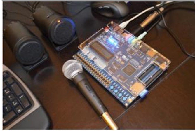
Figure 9.1: Project setup including speakers, mic and DE2 board connected to the computer [5]
