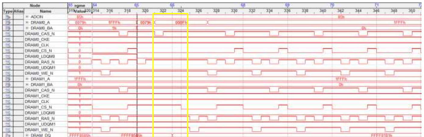
Fig. 14. Captured waveform of reading data from the SDRAM 1 by using SignalTap II
