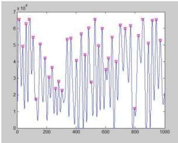
**Figure-16.** Detected peak results from the “findpeaks” command and results from the microprocessor system.
