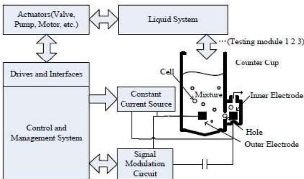
Figure-2. The automatic hematology analyser system [11].
