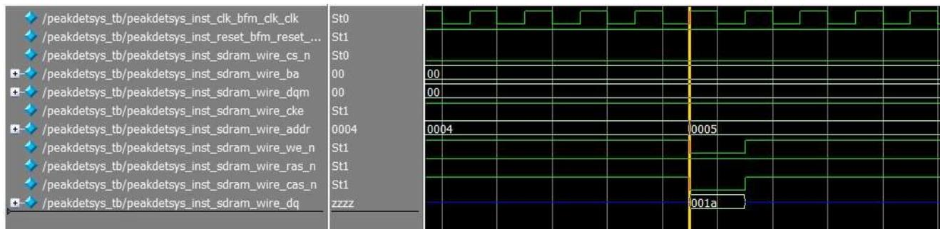
**Figure-15.** Waveform of the write operation on SDRAM memory location 0x0005, with value 0x001A.
