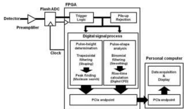
Figure-4. Block diagram of the digital signal processing system for radiation spectroscopy [5].
