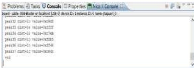
**Figure-17.** Results of detected peak display in the Nios II console.
