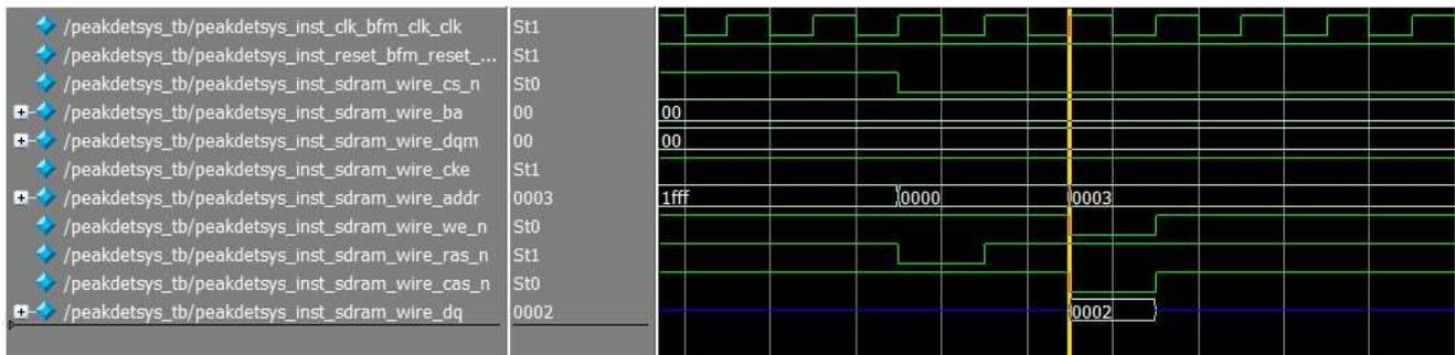
**Figure-13.** Waveform of the write operation on SDRAM memory location 0x0003, with value 0x0002.
