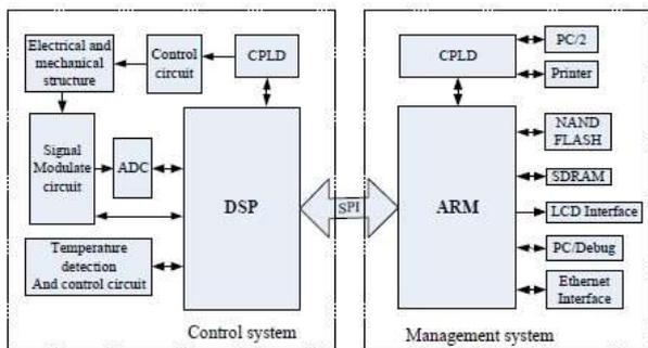
Figure-3. Block diagram of the embedded system design for automatic hematology analyser [11].
