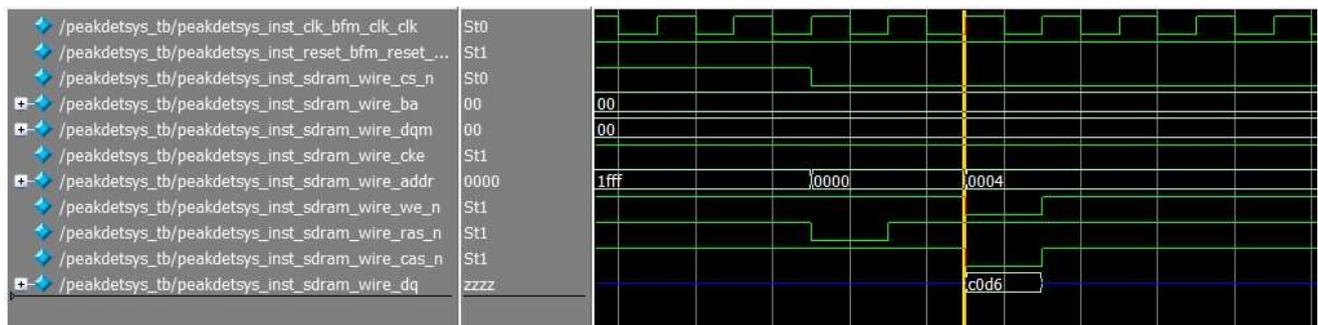
**Figure-14.** Waveform of the write operation on SDRAM memory location 0x0004, with value 0xC0D6.
