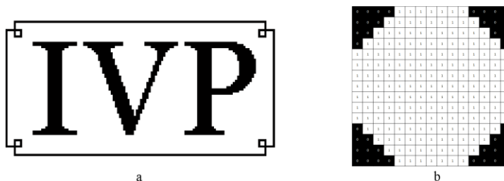
Figure 1: (a) Input image [15], (b) structuring element of a disk shape with a radius of eight pixels
