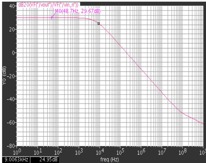
Fig. 6: Results of AC analysis for the telescopic op-amp
