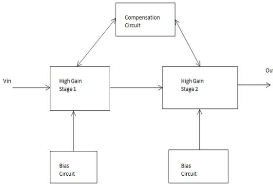
Fig. 1: Two-stage CMOS op-amp
