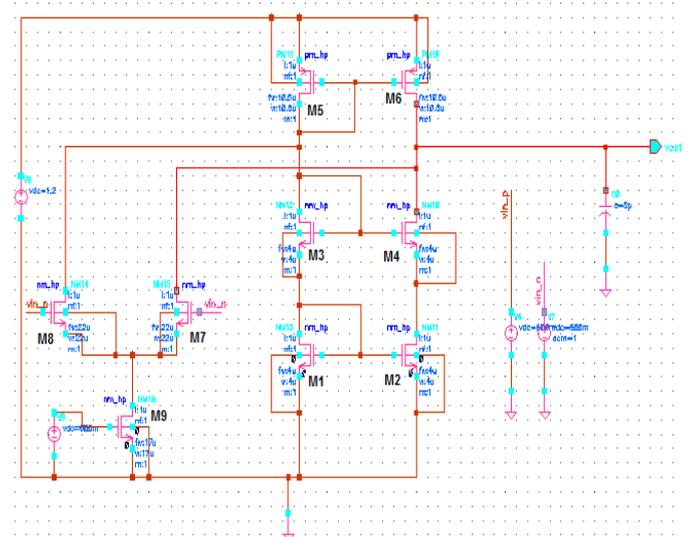
Fig. 4: Op-amp topologies: folded cascode
