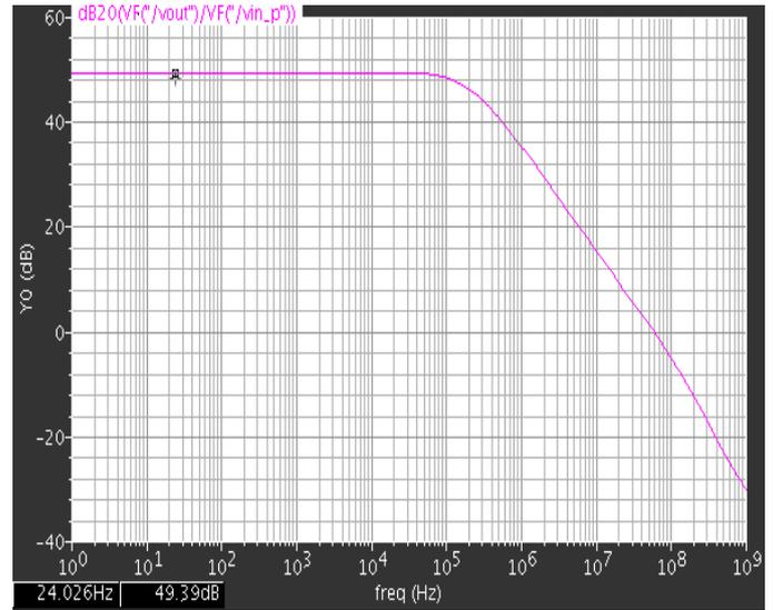
Fig. 7: Results of AC analysis for the folded cascade op-amp
