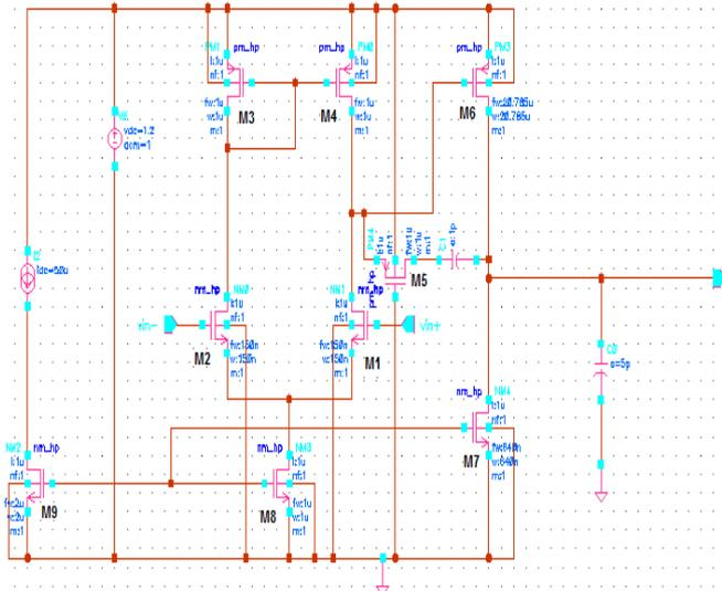
Fig. 2: Op-amp topologies: two-stage
