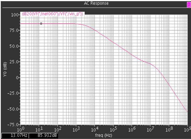
Fig. 5: Results of AC analysis for the two-stage op-amp
